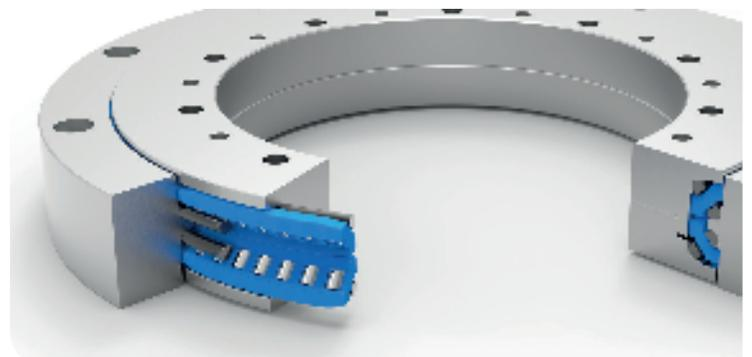
and thus increase the load capacity of the bearing by up to 50% compared to ball bearings. Due to the crosswise arrangement of the rollers, the same high loads can be absorbed from all directions.
