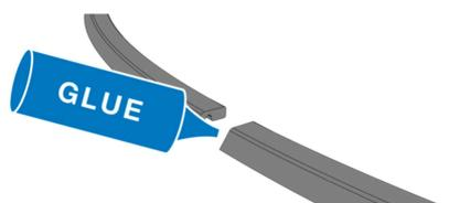
Fig. 34: Coat parting points with adhesive
