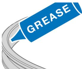
Fig. 9: Lubricate wire
