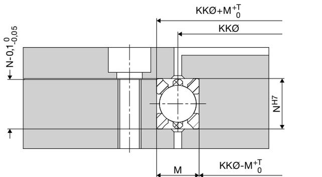
The statements made in the section for LEL apply to the constructive design. The wire bed has no radii to accommodate the race, but the tool radii must not exceed 0.2 mm.
