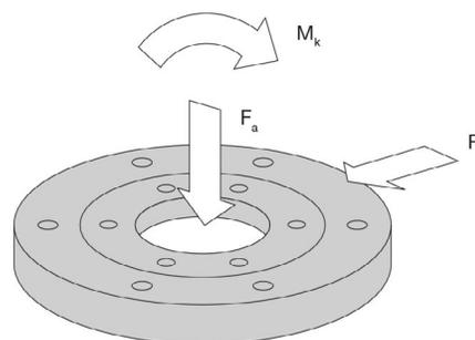
All forces and moments acting on the bearing are to be combined by vectorial addition into centrally acting forces  $F_a$  and  $F_r$  and resulting moments  $M_a$ . For complex load cases and load spectra with variable loads and speeds, we will be pleased to calculate the values for you.
