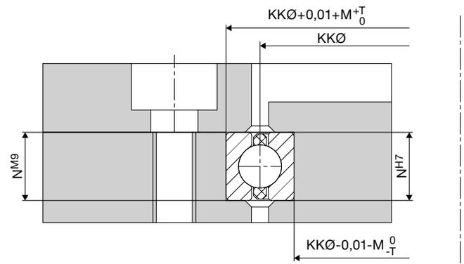
The wire bed has no radii to accommodate the race, but the tool radii must not exceed 0.2 mm.  $T = 0.03$  mm for KK up to 300 | 0.04 mm for KK greater than 300 (mm).
