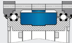
1. Franke-Torque with water cooling, KKØ 300mm
