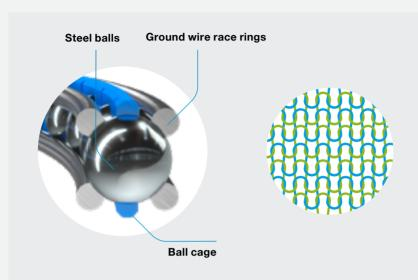
The bearing that rotates the dial, cylinders and fabric take-down has the biggest influence on the needle guidance and therefore on the fabric that is produced. Perfect results are only achieved by accurate radial and axial guidance of the needles. The introduction of Franke bearings as component parts has become a pioneering development in the design of high-performance circuar knitting machines.
